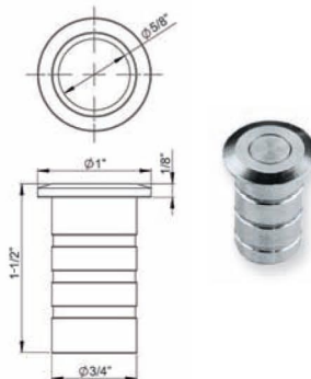
DBIX901 / DBIX902 Dust Proof Floor Bolt Strike Stainless Steel Dia. 13.5mm for Dia.13mm Bolt Dia. 11.5mm for Dia. 11mm Bolt Face Plate Screws included
